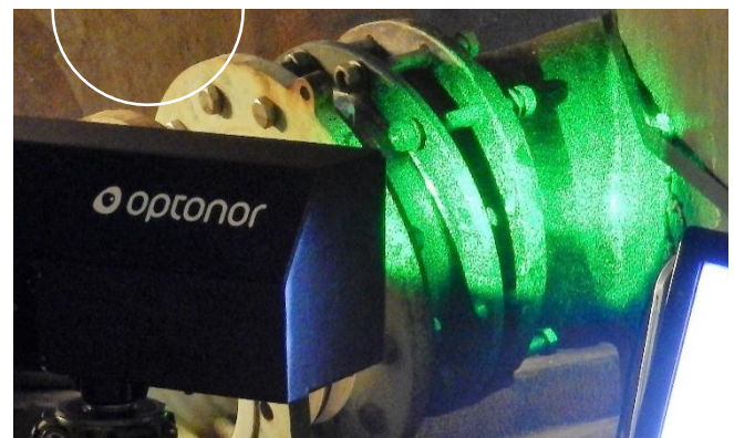
Fig 5. Complex geometries are inspected by the non-contact, camera-based system.
